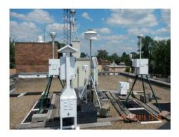
Site description: This is a source oriented FRM  $PM_{2.5}$  site located near the Canton Timken plant in SW Canton. The instruments are located on the roof of Canton's Firestation House No. 8. The site has also a  $PM_{2.5}$  chemical speciation monitor and a carbon speciation monitor. This is a suburban location setting and the land use is considered industrial/residential.
